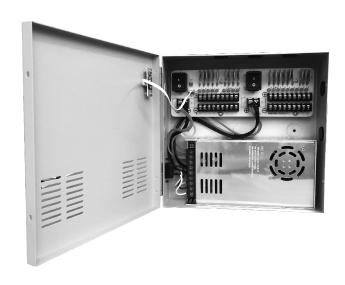
The OE-1230AD18 is a cost effective way to power up to 18 cameras in a security system. Individual class PTC fuses for each output as well as over current voltage protection that provides a high level of protection.
